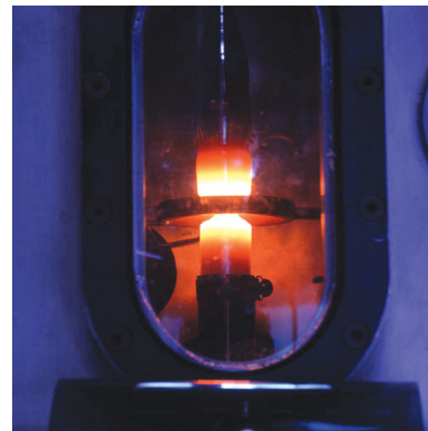
A silicon crystal takes shape using the float-zone refining method. photo: NREL PIX and Jim Yost Photography
