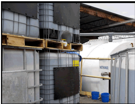
Fig. 1 - Tanks of methanol and tubs of glycerin, the byproducts of biodiesel production, are stored in safer areas outside Foothills Bio-Energies before being removed by tanker or truck.
