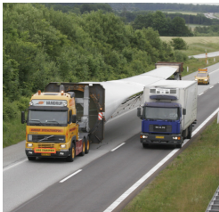
Fig. 6 – A 200-foot blade for a 5MW offshore turbine being transported to Scotland
